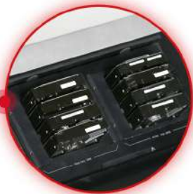
Write-block hard disk (SATA/SAS) slots
