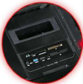
Write-block ports (IDE/SATA/USB/Memory Cards)
